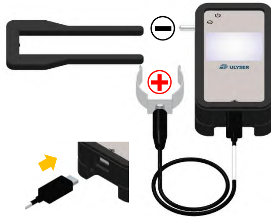
Figure 11: Setup for measurement of ULD types with one water switch pin
