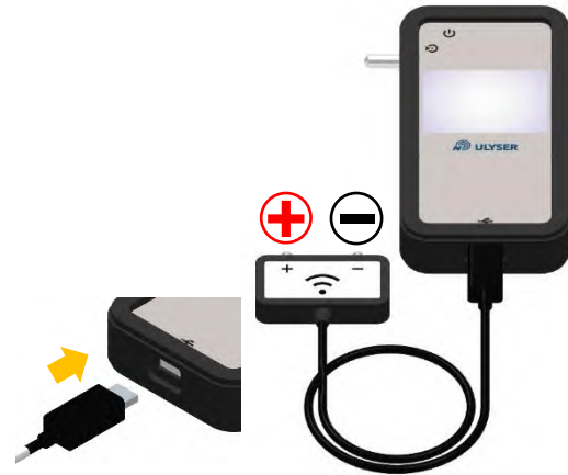
Figure 13: Setup for measurement of LF-ULD types with two water switch pins
